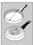
Some saucepans have a smaller ferromagnetic area than the real diameter of the saucepans. Only this area will be heated up by the induction zone. therefore the cooking performance may be reduced These pan types cannot be detected by bigger induction zones. The diameter of pan's ferromagnetic area should match the size of the cooking zone. If the pan is not detected by the cooking zone, try it on the next smaller cooking zone.
