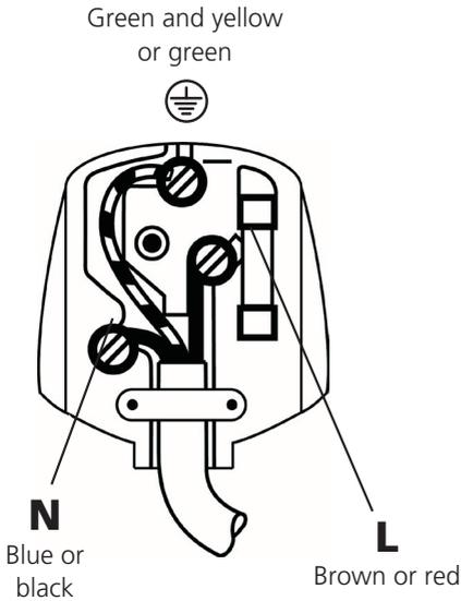
With the alternative plugs a 13A fuse must be fitted either in the plug or adaptor or in the main fuse box. If in doubt contact a qualified electrician.
