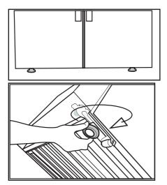
To adjust the doors vertically, Loosen the fixing nut located at the bottom.
