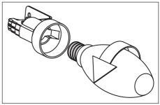
Fig. 14: Replacing the spark plug lamp
