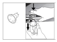
Fig. 13: Replacing the LED lamp
