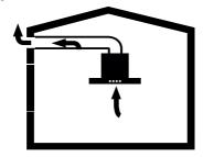
Fig. 4: Exhausting the air without a carbon filter
