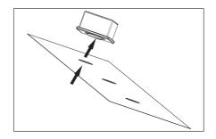
Fig. 15 Replacing the LEDs
