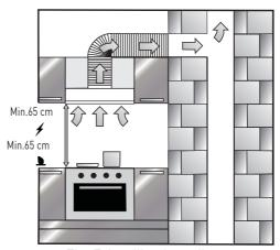
Fig. 7 Installing the appliance
