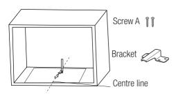
3. Remove the bottom cabinet template and fix the bracket with screw A.
