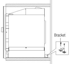
Open the door, fix the oven to the cabinet with Screw B through the installation hole. Then fix the trim-kit plastic cover to the installation hole.
